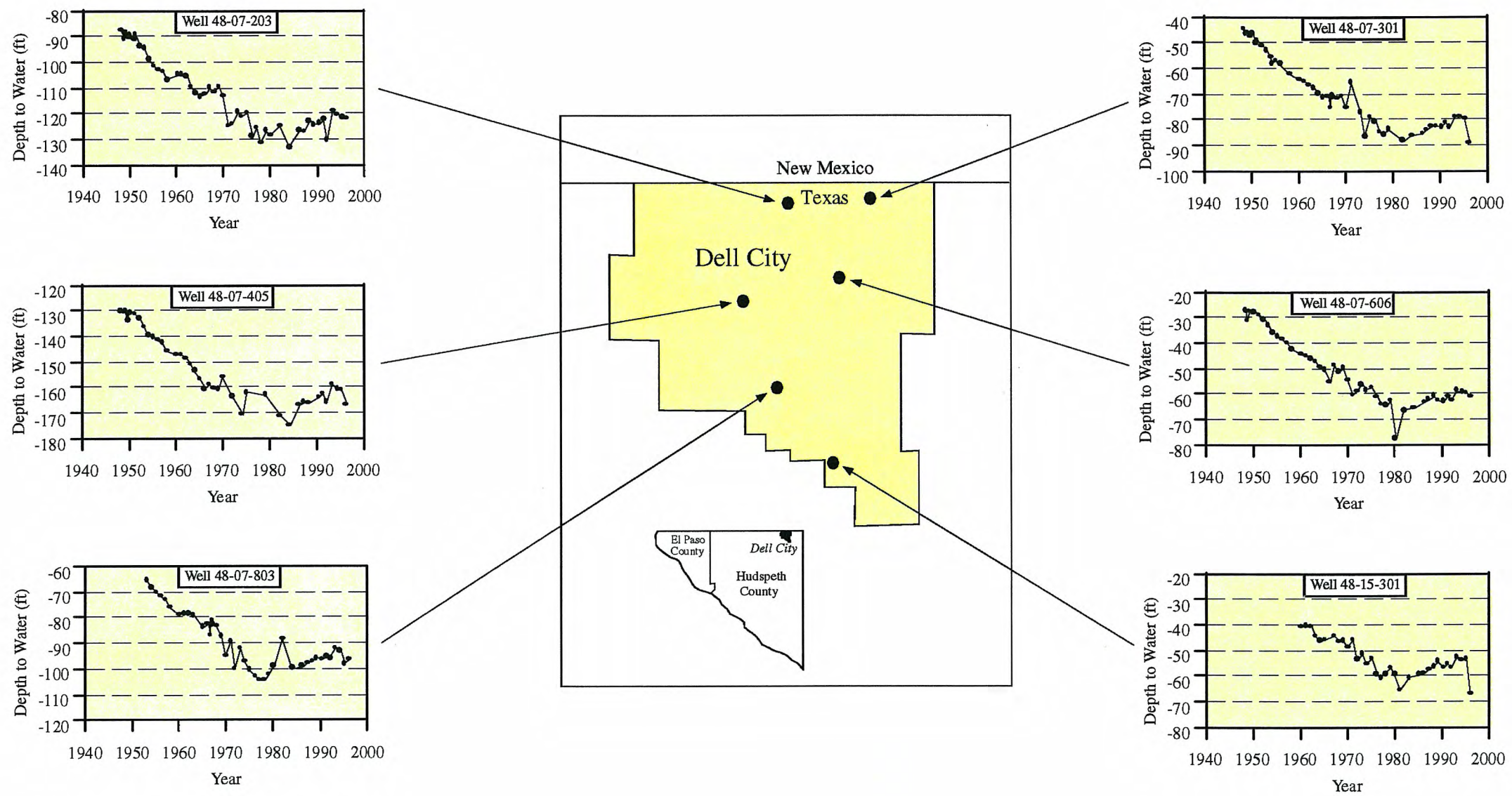
Figure 6.3. Hydrographs of selected wells in the Dell City area (modified from Ashworth, 1995).
