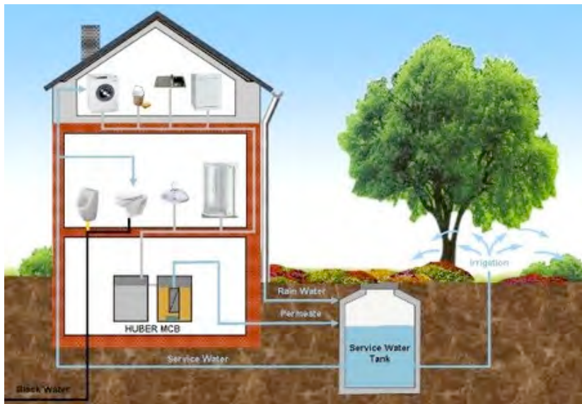
Figure 4.2. Illustration of a household gray water system.
