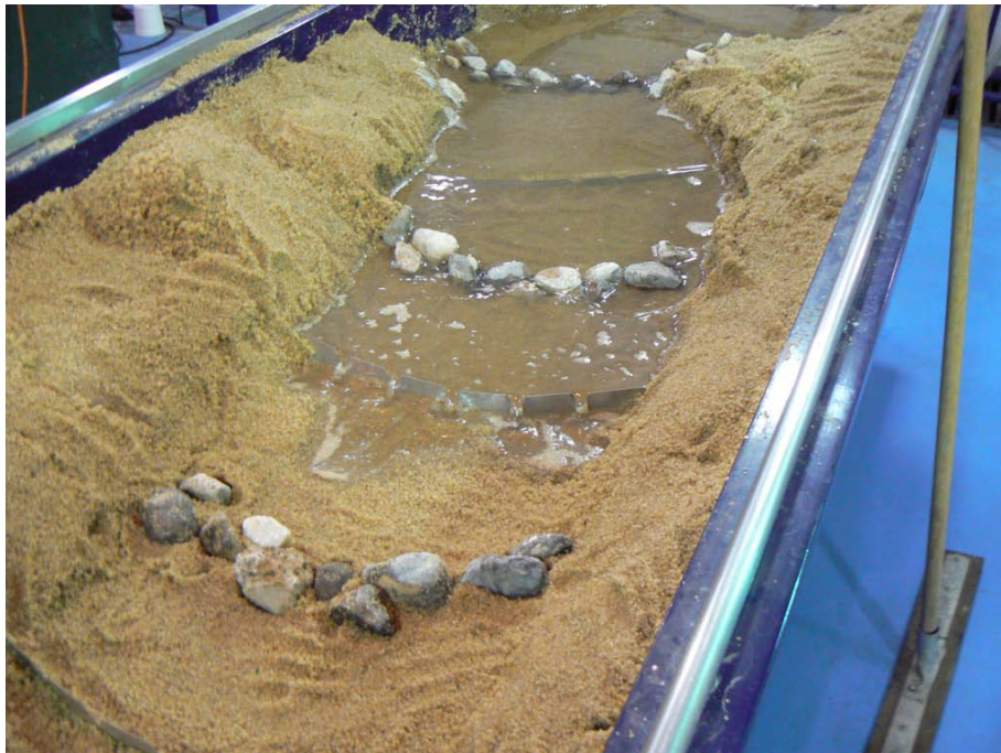
Figure 14 Scale Model Check Dam Performance 10 Year
