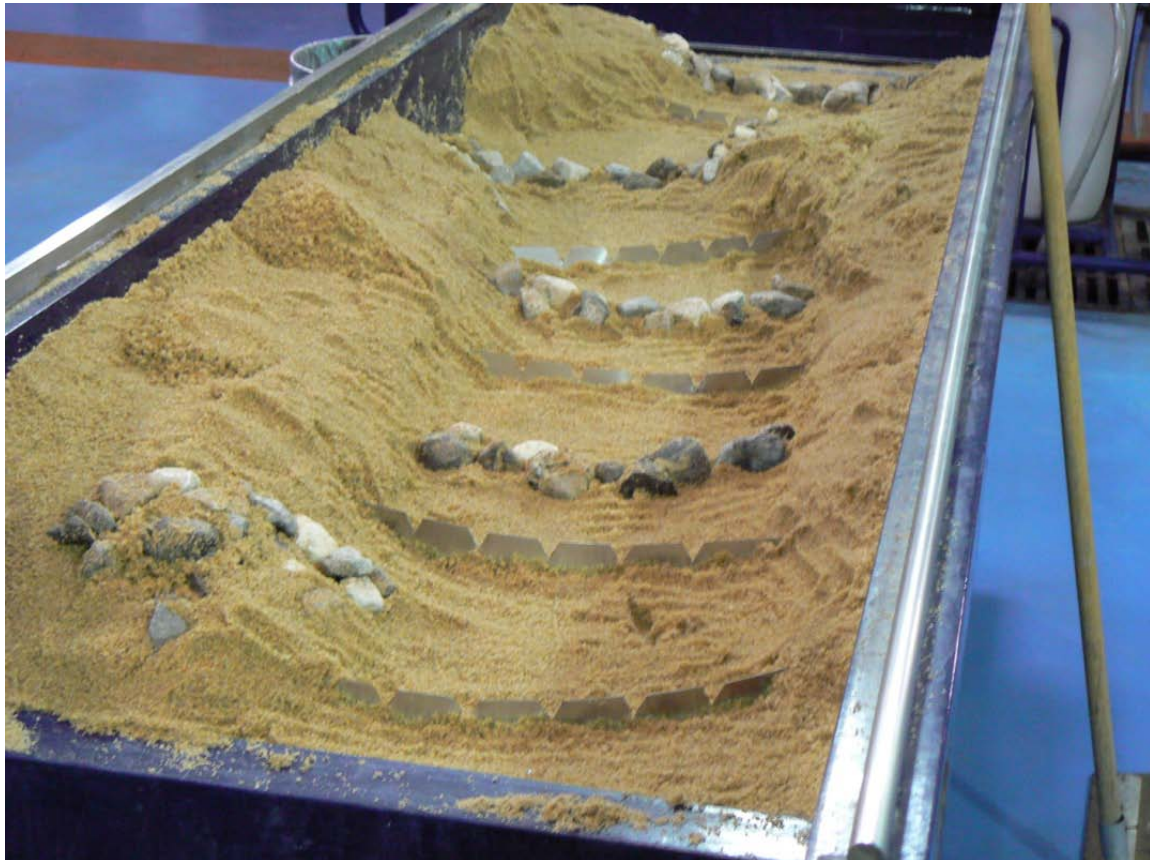
Figure 12 Scale Model of Center Channel for Testing
