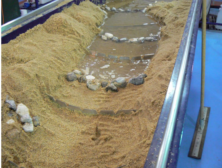
Figure 14 Scale Model Check Dam Performance 10 Year
